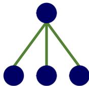
The **type-of relation** is used to create classes of systems and system elements. This is used for recognition of the systems and to prevent information from “growing wild”. This is what the classes in 81346-2 is about.
