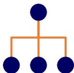
The **part-of relation** is used to sub-divide any system into its constituent parts, recognised as system elements. This enables unlimited subdivision of complex systems and this is what 81346-1 is about.
